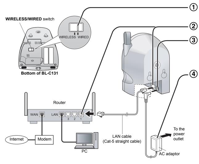
**BL-C131 only:** Confirm that the WIRELESS/WIRED switch on the bottom of the camera is set to **WIRED**.
