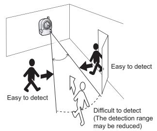
**6.** If the lens is aimed at an area outside of the sensor's active detection range, the objects that trigger the sensor may not be visible, and therefore buffered or transferred images may not show the object that triggered the sensor.
