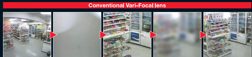
Defocusing when field of view is changed. Awkward setup on IP cameras with image latency.
